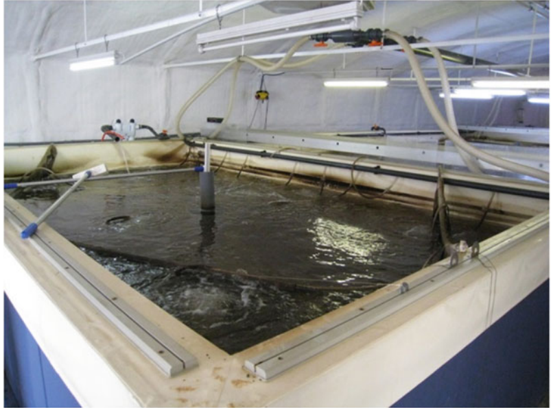
Fig. 6.28 Intensive indoor shrimp production in a recirculating aquaculture system in Germany (Photo: J. Pucher)
